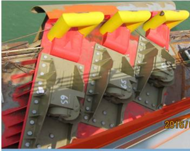
Chain Stoppers of 12 Point Mooring System Installation
